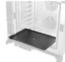
Cooking fat and liquid collection kit: non-stick stainless-steel container h 20mm, designed with special bendings and a central hole to collect liquids and fat dripping from the food and direct them to the center of the drain to reduce the dirtiness on the cooking chamber. Strongly recommended with SMART.Drain and in any dirty intensive cooking of poultry and meat.
