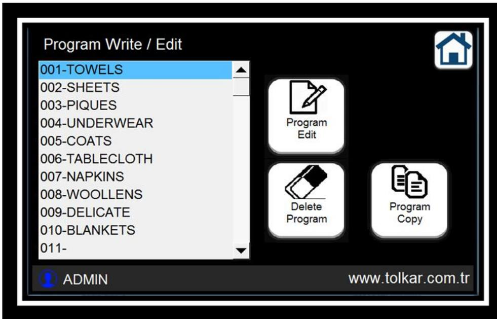
Pressing the button “PROGRAM DÜZENLE” (EDIT PROGRAM) on this screen, displays the the content of the selected program. This page contains the parameters to be applied by the machine when operating in heating phase.
