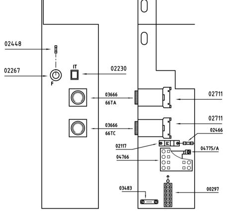
IMPIANTO ELETTRICO PER MACCHINA CON CALDAIA (DISPOSITIVO A 220 VOLTS)
